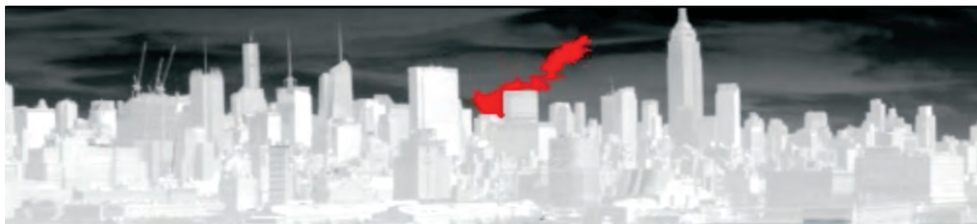
Plume of HCFC-22 detected by M. Ghandehari et al (2017) using a ground based, long-wave infrared (LWIR) hyperspectral imaging (HSI) sensor.
