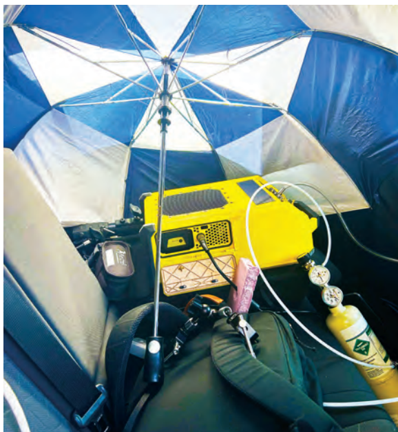
(Clockwise): Observing Gasmeter detection readings in the field; Gasmeter probe extended on pole, collecting air readings; Gasmeter device and equipment for maintaining stable baseline for data collection.
