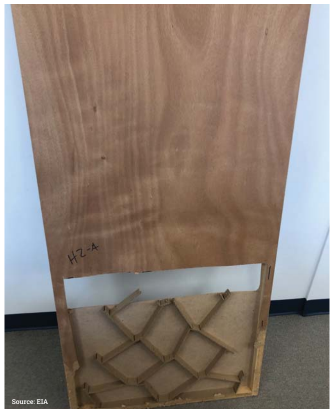
Figure 3 Structure of the Jeld-Wen door
