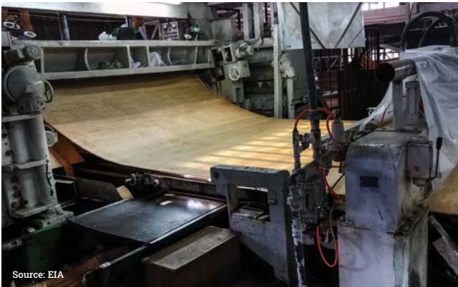
Figure 5 Peeling of okoume log in China
