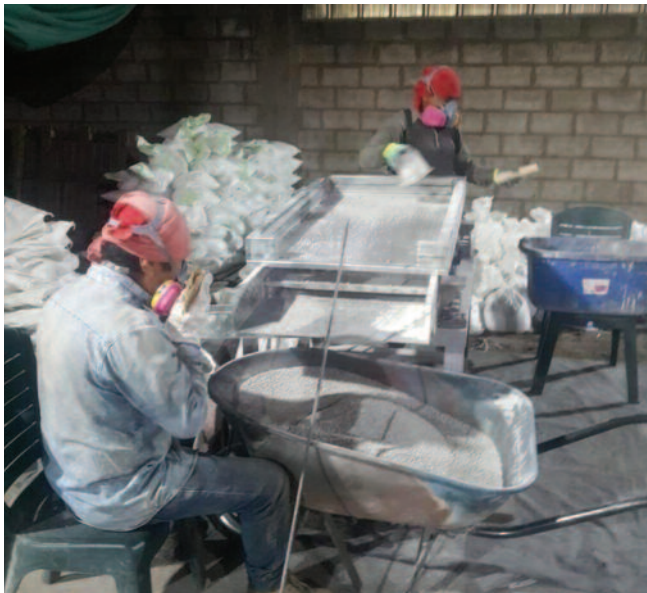
Figure 27 Processing of mercury-laden gravel, filtering (left) and washing (right)
