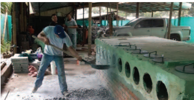
Figure 28 Second phase of extraction by combustion
