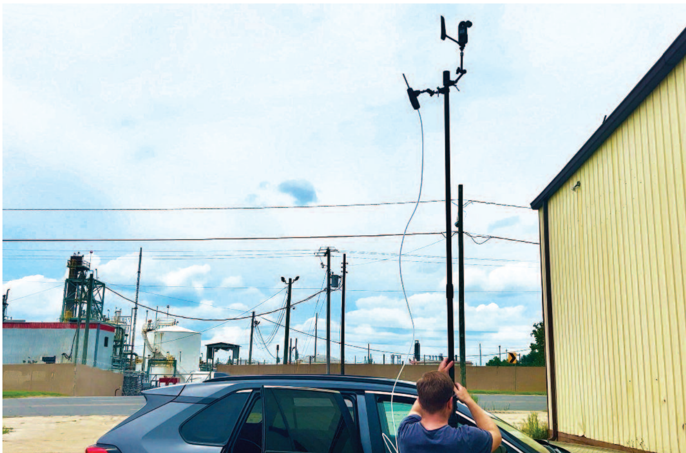
EIA investigator setting up infrared detection equipment outside Honeywell International's fluorochemical facility at Baton Rouge, Louisiana, USA. EIA investigators detected an array of fluorinated gas emissions from the fenceline of the facility, including several CFCs and HFCs not reported by the facility in recent years of mandatory greenhouse gas and toxic substances reporting. 33
