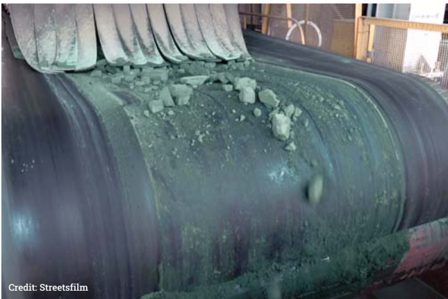
Figure 6 Cobalt hydroxide belt at TFM
